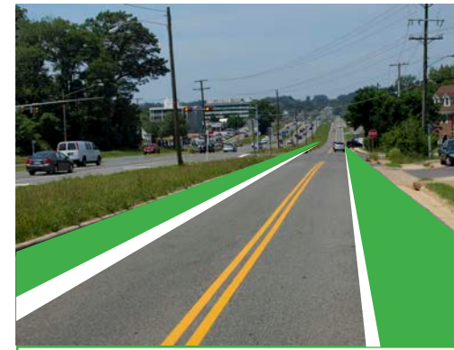
This service road has room for cars and protected bicycle lanes (South Street, north side)
